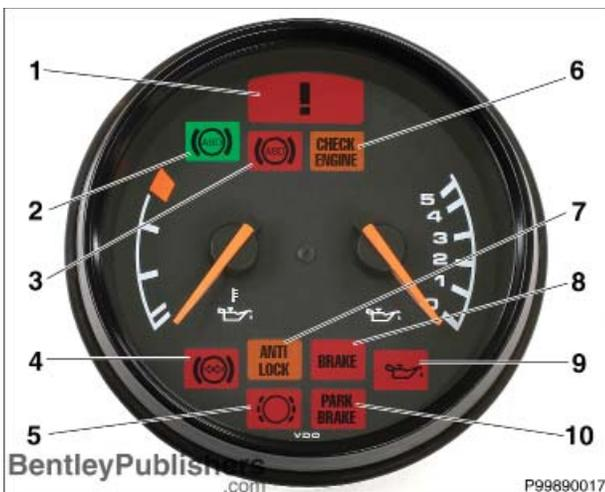
The central warning light and individual warning lights come on momentarily when ignition is switched ON. If a fault occurs, the central warning light comes on with the corresponding warning light(s). The cancel button in the center console can be used to cancel the central warning light.
